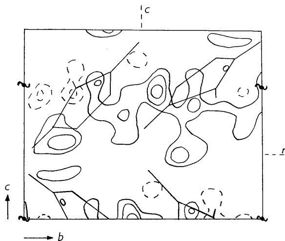
Fig. 3. The 0kl (F_o - F_c) synthesis showing the positions of the hydrogen atoms in the hydrogen bond. Contours every 0.25 \text{ e.}\text{\AA}^{-2} .
